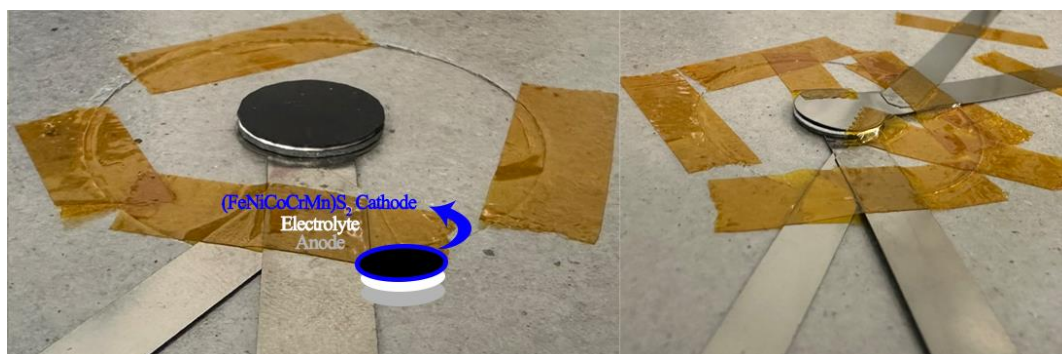
Figure 3.7. The single cells containing (FeNiCoCrMn) S_2 high entropy disulfide cathode.
