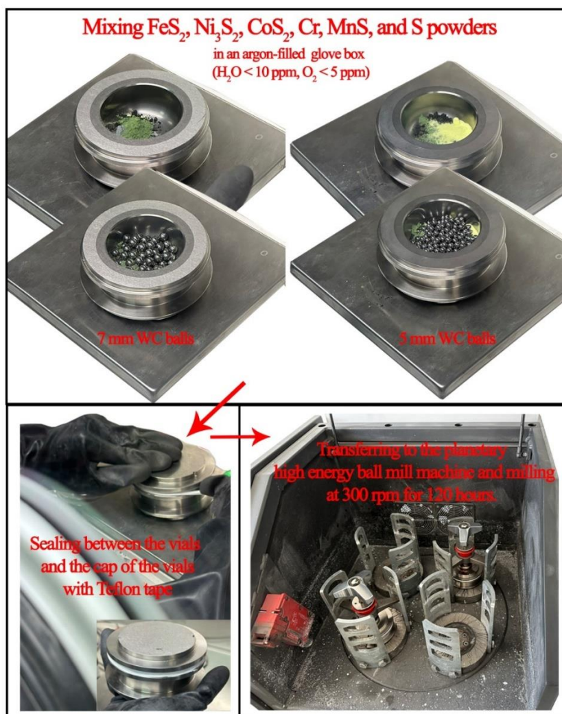
Figure 3.5. Ball milling procedure performed to synthesize (\text{FeNiCoCrMn})\text{S}_2 high entropy sulfides.
