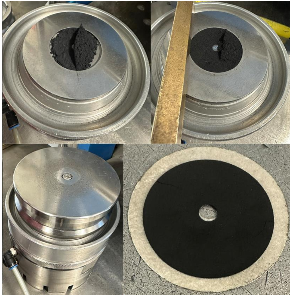
Figure 3.6. Preparing of the (\text{FeNiCoCrMn})\text{S}_2 pellets with 40 mm diameter.
